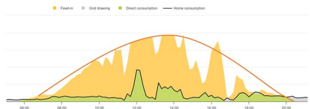
Fig. 2 PV Plant typical production diagram (Source: Innerga)
